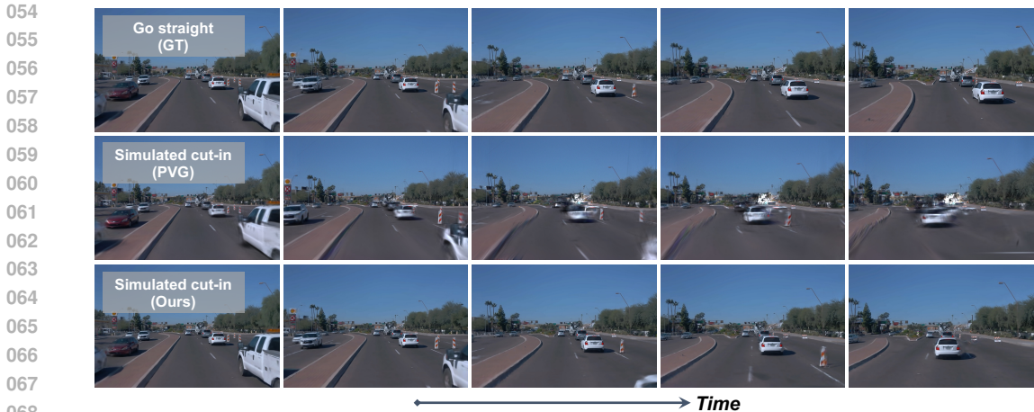
Figure 1: We simulate a cut-in case in a high-speed scenario, which is a typical functionality in driving simulators. The representative method PVG (Chen et al., 2023) fails after the lane change. We provide more video demonstrations in the attached supplementary materials.
