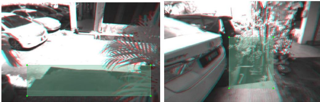
Figure 8: Examples of bounding box annotation on the anaglyph of two different samples - down-steps (left) and uncovered drainage (right).
