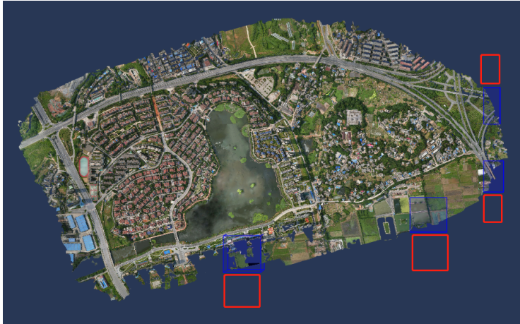
Figure 10: Blank Tile Distribution Chart (as indicated by the red box in the image).
