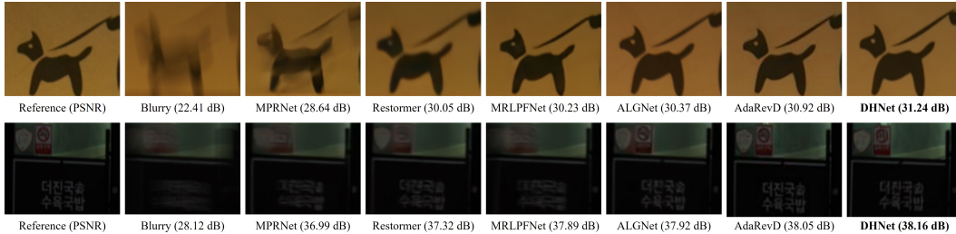
Figure 11: Comparison of image motion deblurring on the RealBlur dataset Rim et al. (2020).
