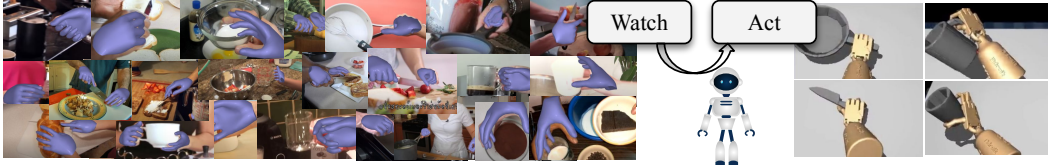
Figure 1: Main idea: We learn dexterous grasping by watching human-object interactions in YouTube how-to videos. Using hand poses extracted from a repository of curated human grasp images (left), we train a dexterous robotic agent to learn to grasp objects in simulation (right). The key benefits include improved grasping performance and the ability to quickly scale the method to new objects.
