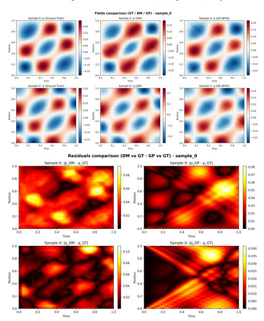
Figure 5: Validation of GP-dPHS performance and PHDME performance. The left column is the ground-truth dynamics generated by A.1, the middle column is the forecast made by the proposed method, and the last column is the GP-dPHS prediction based on the initial conditions. Key takeaway: Both GP-dPHS and PHDME have learned the correct dynamic patterns, but not 100% perfect. The red residual comparsion figures show the differences, notice that the magnitude of the residual is very low.
