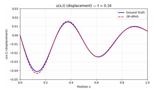
Figure 6: This is the reconstruction based on the derivative field, the blue line is the movement (displacement) of the soft string system using a faithful physics simulator. The red dot line is the one reconstructed based on the derivative field using the rollout that has been mentioned above. Key takeaway: The state and state derivative method is applicable to the physics-informed machine learning.
