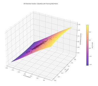
Figure 8: GP-learned representation of dE/dq (partial derivatives of energy) with training data points. The limited observations lie on the surface of the GP plane, indicating the correct and smooth energy representation of the system.
