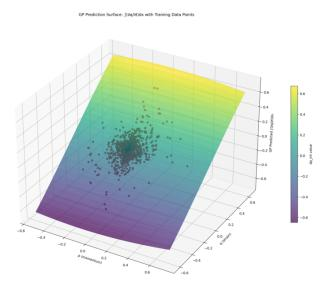
Figure 7: GP-learned representation of dE/dp (partial derivative of energy) with training data points. The limited observations lie on the surface of the GP plane, indicating the correct and smooth energy representation of the system.
