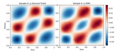
Figure 4: Left: Ground-truth state evolution of the wave equation. Right: Physically consistent and accurate prediction of PHDME based on sparse data and limited knowledge of the governing equations. Key takeaway: PHDME generates samples with correct dynamic pattern and amplitude by only conditioning on the initial two frames.
