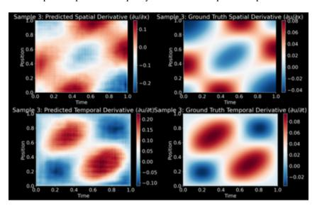
Figure 9: The left side is the dynamic generated by the data-driven diffusion model, while the right side is the ground truth dynamics generated by the physically-faithful simulator. It's obvious that the pure-data-driven method compromises its accuracy under the initial conditions that have never been met before.
