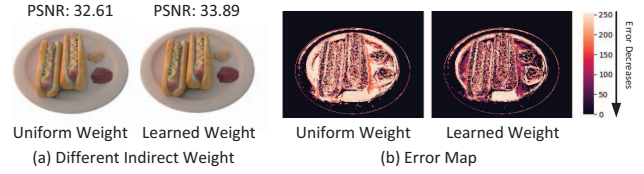
Figure 4. Environment Weight. We visualize rendering results and their error maps with uniform and learned weights.
