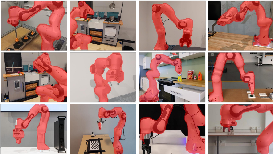
Figure 15: Segmentation masks predicted on out-of-distribution images by a fine-tuned Mask-RCNN model (He et al., 2017).
