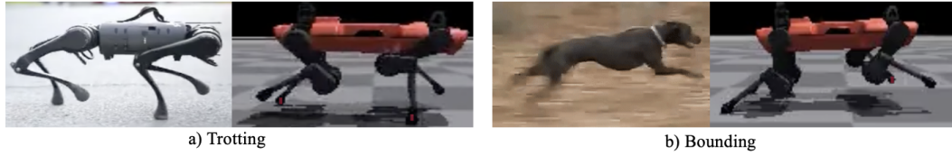
Figure 11: Demonstration of the generalization capabilities of SDS on the ANYmal quadruped robot, featuring an inverted joint configuration and significantly different kinematics. Comparison between demonstration and learned behavior frames for a) trotting and b) bounding skills. (Red corresponds to left-side legs)
