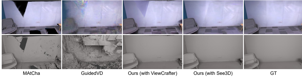
Figure A8: Qualitative comparison from 5 input views using different diffusion models. G4Splat produces high-quality, smooth geometry reconstruction even when paired with a weaker generative prior, and it continues to effectively suppress Gaussian floaters and reduce blurriness in the rendered results.
