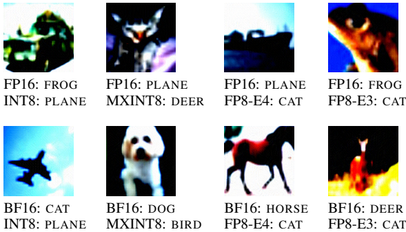
Figure 4. Example border images of MobileNet-v3-Small generated by HSPI-BI. The predicted label changes when fed to the same model quantized to different number formats. The subcaption follows the format of model format : predicted label.
