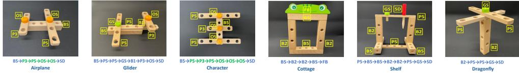
Figure 3: Visualization of building block assembly tasks, with objects labeled in yellow. Each task is accompanied by a workflow outlining a correct sequence of operations required to complete the task. Objects highlighted in green can be rearranged in different orders.
