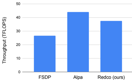
Figure 6: The comparison of throughput in the running of GPT-J-6B on a 4 \times A100 server.
