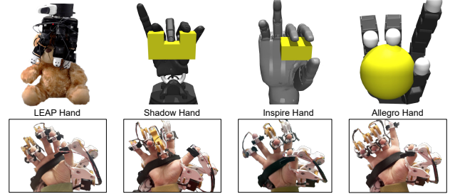
Fig. 4: Action retargeting results: Teleoperating the LEAP Hand to grasp a toy in the real world and teleoperating the Shadow Hand, Inspire Hand, and Allegro Hand in simulation.
