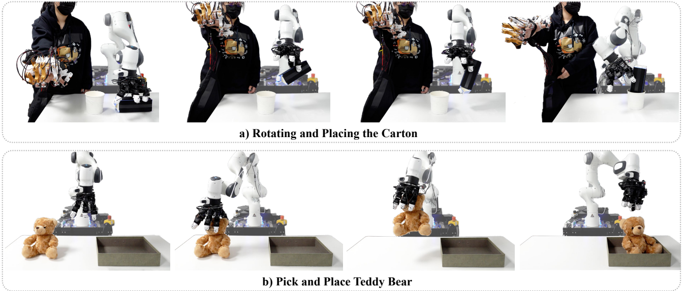
Fig. 5: (a) Teleoperation experiment : In in-hand rotation, the challenge is to slightly release the fingers, allowing the carton to rotate without slipping out (as shown in the middle two images). (b) Imitation learning evaluation : The robot must first locate the bear, then open its hand to grasp it. Due to the bear’s size, precise grasping control is required. An inaccurate grasp deforms the bear and causes it to slip out of the fingertips.
