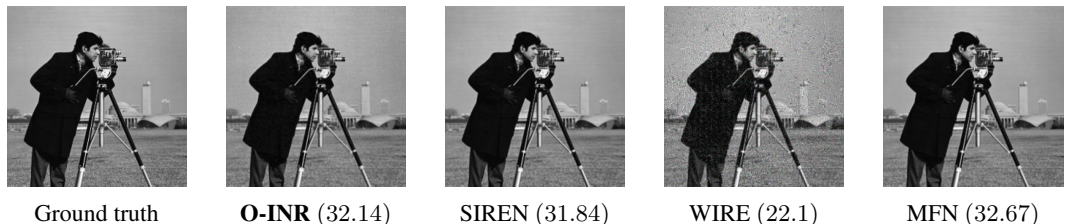
Figure 10: Performance comparisons of O-INR in multi-resolution training setting. The ground-truth together with images from O-INR and other baselines (L to R), with the PSNR value in dB. O-INR achieves comparable/better performance
