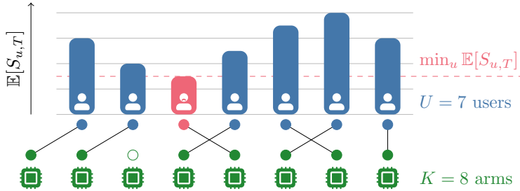
Figure 1: An illustration with K = 8 arms and U = 7 users. After time step T , each user u \in [U] has some expected cumulative reward \mathbb{E}[S_{u,T}] . The agent’s objective is to maximize \min_{u \in [U]} \mathbb{E}[S_{u,T}] , which is the minimum expected cumulative reward across all users.
