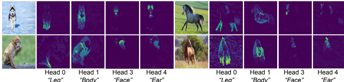
Figure 7: Visualization of semantic heads. We forward a mini-batch of images through a supervised CRATE and examine the attention maps from all the heads in the penultimate layer. We visualize a selection of attention heads to show that certain heads convey specific semantic meaning, i.e. head 0 ↔ "Legs", head 1 ↔ "Body", head 3 ↔ "Face", head 4 ↔ "Ear". See more in Figure 15
