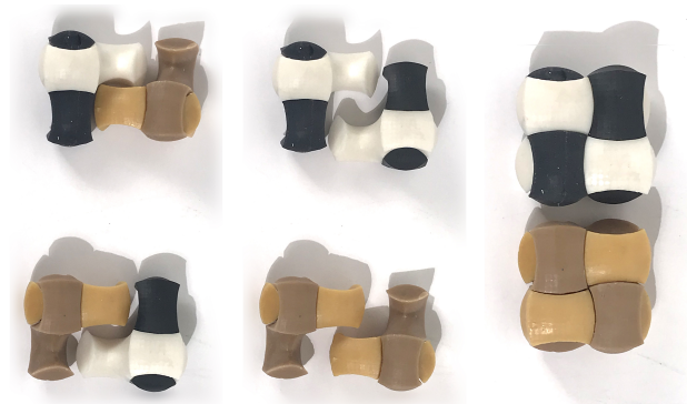
(a) Chiral pairs of plain (b) Pairs belonging to the (c) Plain woven assembly of two chiral groups. same chiral group can be assembled.
