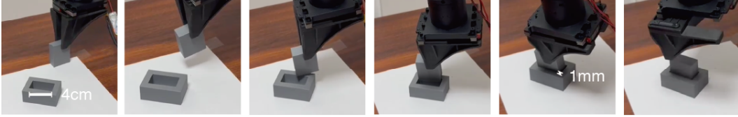
Figure 7: A rollout of fine-grained insertion. Our method can achieve high precision, even if we are observing the motion from 40cm away without a wrist camera. However, we observe an adjustment behavior resembling bang-bang control – it is still challenging for the policy to insert accurately in one-shot as human. Fortunately, it still captures rough directions for adjustment to finish the task.
