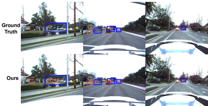
Figure 5: Detected unlabeled objects. The first line is the 3D box of the ground-truth, and the second line is the detection result predicted by our algorithm. The blue box indicates that our algorithm can detect some unlabeled boxes. Please zoom in while maintaining the color.
