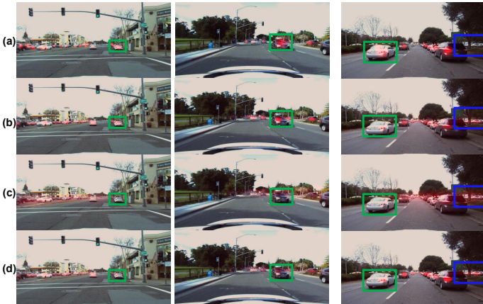
Figure 3: Visualization of heatmaps on target domain: (a) ground-truth, (b) 2D detector, (c) rendered from IVF, and (d) revised by 2D detector. The green rectangles indicates that our algorithm has improved the confidence of the detector prediction. The blue rectangles represent unlabeled objects that our algorithm detects. Please zoom in while maintaining the color.
