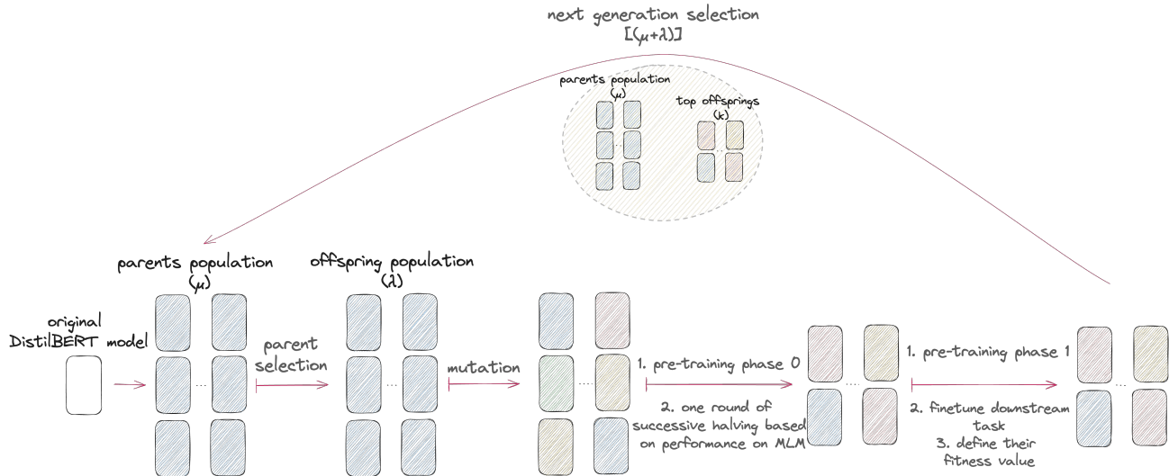
Figure 1. The NAS pipeline outlines the operational steps for the proposed exploration method, based on genetic algorithms. The original DistilBERT model undergoes mutations to create the initial parents’ population of size \mu . Parent selection is then performed by investigating the Pareto front to choose the best-fitted parents. These selected parents undergo further mutations to generate the stemmed offspring population, which requires pre-training. Candidate models are pre-trained, and the top-performing half is chosen based on their masked language modeling loss. Subsequently, the selected models undergo additional pre-training and fine-tuning. Finally, we compute their objective scores and choose the next-generation parents through plus-selection.
