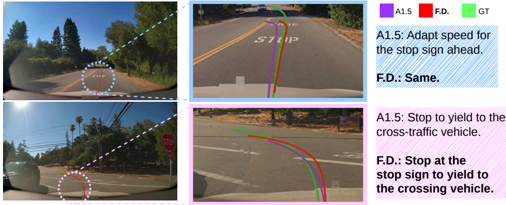
Figure 6: Qualitative comparison of trajectories and CoC results. ( Left ) shows the action visualization, ( Right ) illustrates the corresponding CoT comparisons (Baseline v.s. FlashDrive (F.D.) ). Two common autonomous driving scenarios are selected for illustration: Longitudinal Straight Driving (Row 1), and Oncoming Vehicle Encounter (Row 2).
