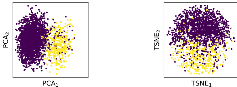
Figure 5: Separability of meta-stable States in latent space. Transforming molecule conformations following the states C_5 and \alpha_R into the latent space, and plotting them in 2D with PCA and TSNE. The colors indicate the different conformations.
