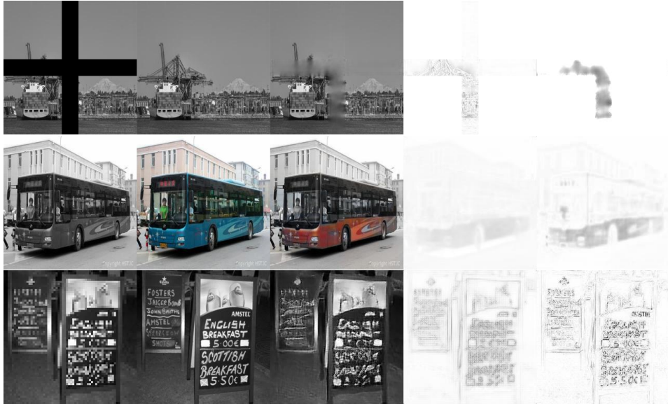
Figure 2: Example of uncertainty masks for image completion (top), colorization (middle) and super resolution (bottom): the images from left to right are the input to the model, the reference image, the output of the model, the calibrated uncertainty mask trained on the L1 loss and the L1 distance heat-map. In the image completion task the bottom left corner is richer in details and thus there is high uncertainty regarding this part in the reconstructed image. For the colorization task, the clothes and the colored area of the bus are the most uncertain regions respectively as these regions can be colorized with a large variety of colors. In the super resolution task the uncertain regions are around the edges and text while smooth surfaces are more certain parts. Note that the actual error (right most image) is not equivalent to our definition of uncertainty and we only present it as a reference.
