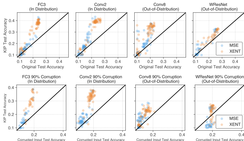
Figure 3: KIP learned images transfers well to finite neural networks. Test accuracy on CIFAR-10 comparing natural images (x-axis) and KIP -learned images (y-axis). Each scatter point corresponds to varying hyperparameters for training (e.g. learning rate). Top row are clean images, bottom row are 90% corrupted images. KIP images were trained using FC1-3, Conv1-2 kernels.
