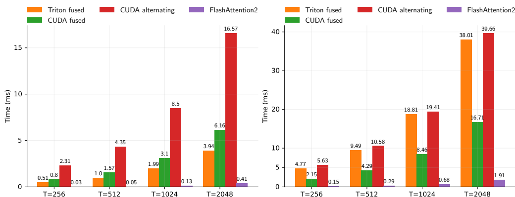
Figure 7: LSTM Runtime for different sequence lengths (T) on a NVIDIA H100. We use 12 heads with head dimension 64 and batch size 16. Left: Forward pass. Right: Forward + backward pass.
