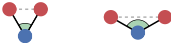
Figure 6: Two different geometric graphs which are undistinguishable from distance edge features, but become distinguishable with angle information between edges or by adding the dashed edge to the graphs.
