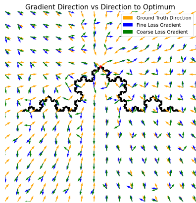
Figure 3. Vector fields illustrating the gradient of error as p_2 is varied in the Koch curve construction, while all other points are held constant at their optimal positions: a) always pointing toward the optimal location (orange); b) the gradient of the fine-scale loss only; and c) the gradient of the multiscale loss. While both gradient vector fields are divergent, the multiscale loss is slightly more aligned with the always-optimal field.
