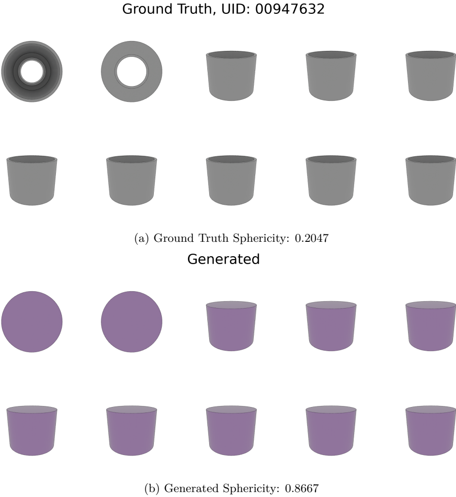
Figure 19: SD : 0.6620; The discrepancy in the sphericity indicates the difference in the overall shape. Higher sphericity indicates closer resemblance to a sphere.
