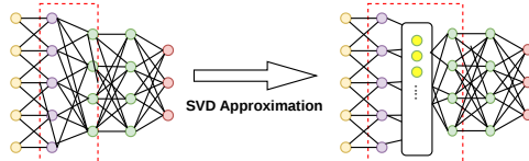
Figure 5: To implement a low-rank constraint, we insert an intermediate linear layer (without activation functions or bias) between the original two layers. This layer acts as a bottleneck that enforces a low-rank factorization of the weight matrix via SVD approximation.
