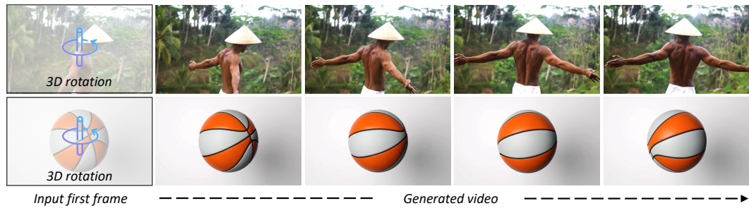
Figure 18: Wan-Move enables object 3D rotation by estimating depth-based positions, applying a rotation, and projecting the results to 2D.
