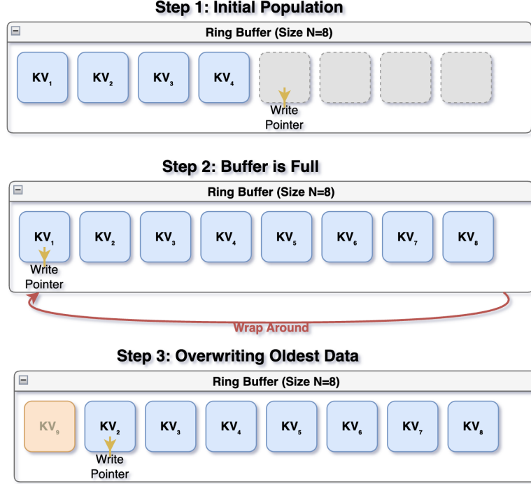
Figure 11: SWA ring-based buffer mechanism. The diagram illustrates the operational lifecycle of the fixed-size ring buffer for KV-cache management in three steps. (1) Initial population: the buffer is filled sequentially, and the attention window covers the active KV pairs. (2) Buffer full: once capacity is reached, the write pointer wraps around to the beginning of the buffer. (3) Overwriting oldest data: a new KV pair ( KV_9 ) replaces the oldest entry ( KV_1 ), ensuring the buffer always contains the most recent tokens while maintaining a constant memory footprint.
