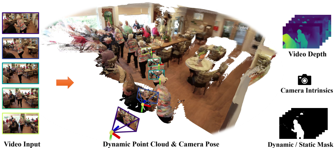
Figure 1: MonST3R processes a dynamic video to produce a time-varying dynamic point cloud, along with per-frame camera poses and intrinsics, in a predominantly feed-forward manner. This representation then enables the efficient computation of downstream tasks, such as video depth estimation and dynamic/static scene segmentation.
