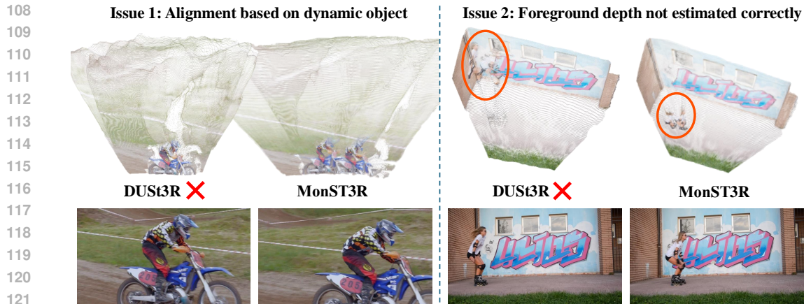
Figure 2: Limitation of DUS3R on dynamic scenes. Left: DUS3R aligns the moving foreground subject and misaligns the background points as it is only trained on static scenes. Right: DUS3R fails to estimate the depth of a foreground subject, placing it in the background.
