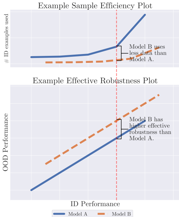
Figure 2: In this schematic example, model B has higher effective robustness and sample efficiency than model A. By plotting OOD performance (effective robustness) and the number of ID training examples used (sample efficiency) against ID performance, we can control for ID performance (vertical slice of plot) to relate sample efficiency to effective robustness.
