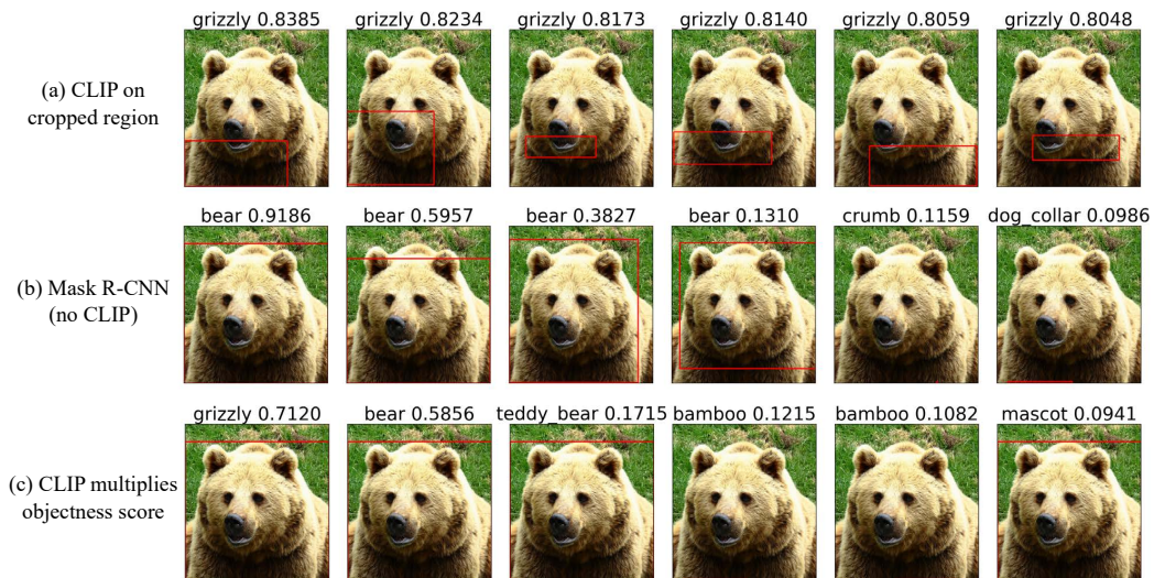
Figure 12: The prediction scores of CLIP do not reflect the quality of bounding box localization. (a): Top predictions of CLIP on cropped region. Boxes of poor qualities receive high scores, though the classification is correct. (b): Top predictions of a vanilla Mask R-CNN model. Box qualities are good while the classification is wrong. (c): We take the geometric mean of CLIP classification score and objectiveness score, and use it to rescore (a). In this way, a high-quality box as well as the correct category rank first.
