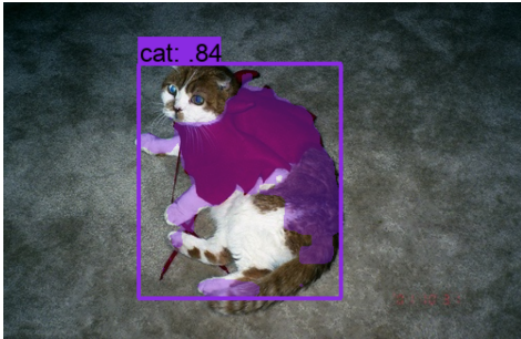
Figure 10: An example of ViLD on PASCAL VOC showing a mask of poor quality. The class-agnostic mask prediction head occasionally predicts masks based on low-level appearance rather than semantics, and thus fails to obtain a complete instance mask.
