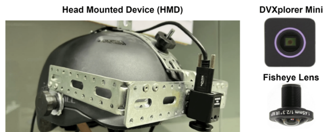
Fig. 5 Our real-world setup. The head-mounted device is equipped with an event camera and a fisheye lens.
