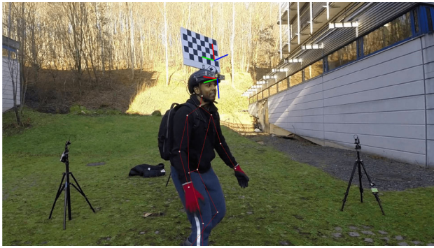
Fig. 19 Visualisation of the Calibrated HMD and 3D human body pose. We employ a multi-view camera setup to simultaneously track the 3D human body pose and the position of a chequerboard in the world coordinate frame. The 3D poses obtained are subsequently projected onto the coordinate frame of the HMD. To establish the coordinate frame of the HMD, we determine a suitable transformation matrix that maps points from the chequerboard’s coordinate frame to the HMD’s coordinate frame. Given the known position of the chequerboard, this transformation matrix allows us to derive the egocentric 3D pose.
