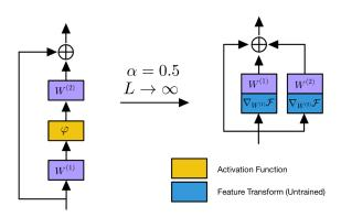
Figure 5: As  $L\to\infty$ ,  $\alpha=0.5$  asymptotically linearizes residual blocks (Eqn. 2). Left: Depth 2 MLP residual block. For  $\alpha=0.5$ , this block is only nonlinear with respect to parameters when L is finite. Right: Linearized MLP residual block, with  $\nabla_{W^{(k)}}\mathcal{F}$  a non-trainable transform of  $h^\ell$ .
