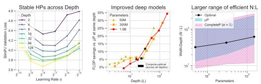
Figure 1: We introduce **CompleteP**, which offers depth-wise HP transfer (**Left**), FLOP savings when training deep models (**Middle**), and a larger range of compute-efficient width/depth ratios (**Right**).
