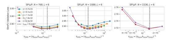
Figure 11: When grid searching learning rate  $\eta_{\text{base}}$  and weight decay  $\lambda_{\text{base}}$ , the optimal  $\tau_{\text{EMA}}$  remains stable.
