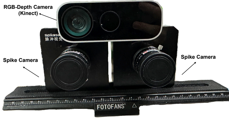
Figure 10: The photograph of our hybrid imaging system. The RGB-D camera is fixed on the top plane of the stereo spike cameras. The extrinsic parameters between the cameras are calibrated.
