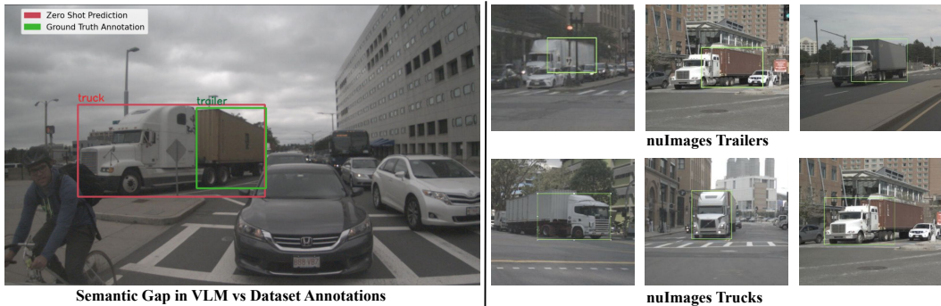
Figure 3: Knowledge Gap between VLM Pre-training and Dataset Annotations. While VLMs show impressive zero-shot performance, they struggle when the concept of the target class is different from vision-language concepts encountered in web-scale training. On the left , we see that the nuImages dataset defines the cab of the truck as a separate object concept from its trailer (shown in green ), while the zero-shot VLM predicts the entire vehicle as a truck (shown in red ). The right visualizes the actual class definitions given to nuImage annotators, provided as both textual descriptions and visual examples. Just as human annotators learn concepts from such few-shot multimodal vision-language data, VLM fine-tuning similarly exploits such multimodal language and visual cues for few-shot learning.
