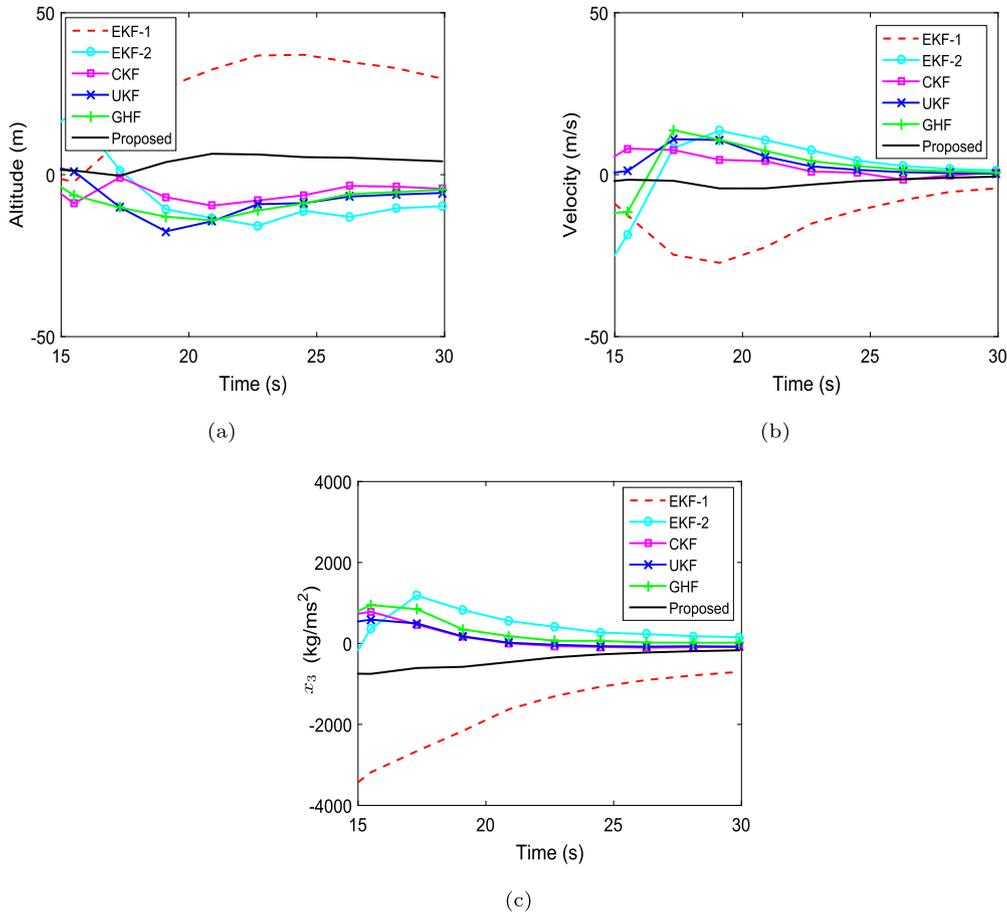
Fig. 4. Mean error vs. time plot for (a) Position (b) Velocity (c) Ballistic coefficient.
