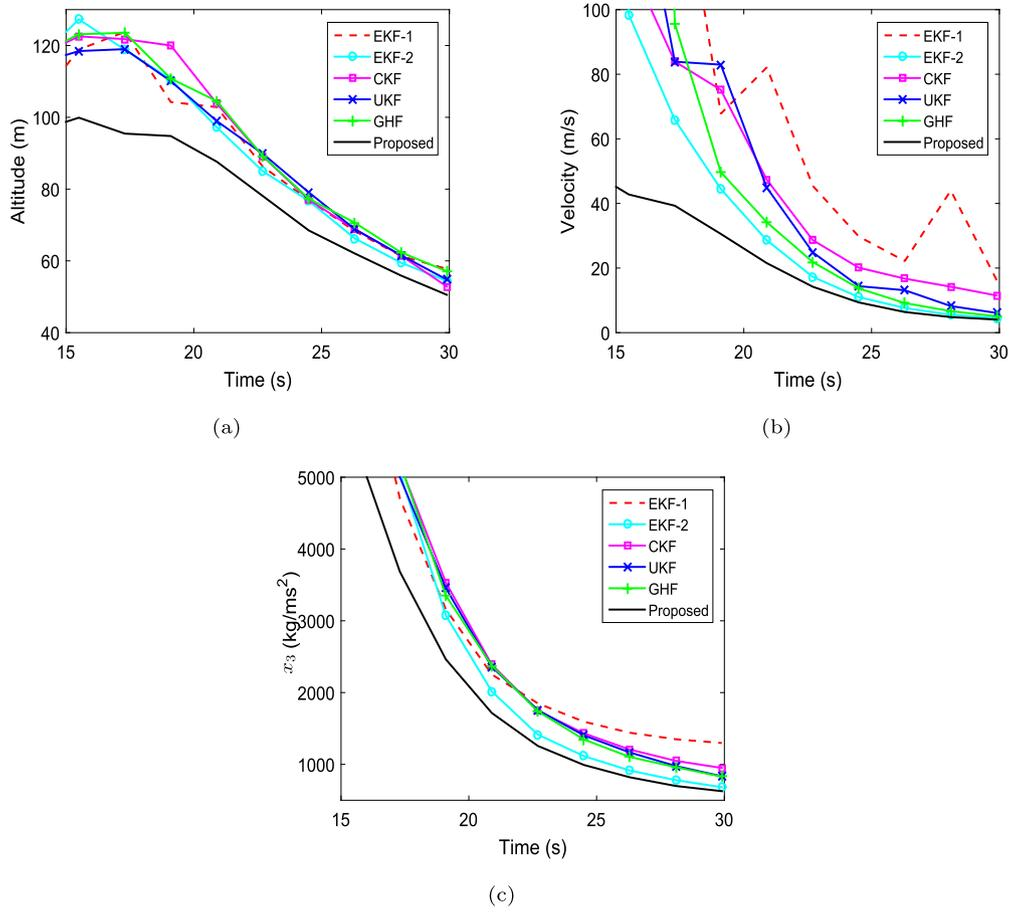
Fig. 5. RMSE vs. time plot for (a) Position (b) Velocity (c) Ballistic coefficient.
