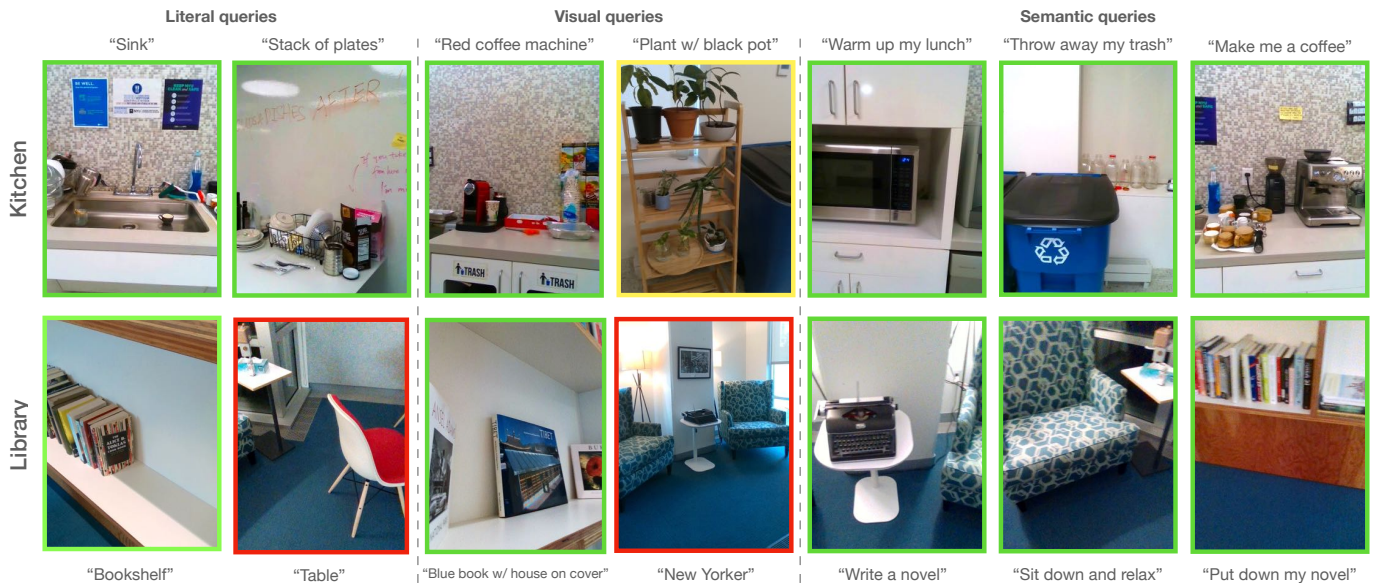
Fig. 3: Examples of the robot’s semantic navigation in two different testing environments, looking at objects given different queries. The images show the robot’s POV given the associated query, with color coded borders showing approximate correctness. The rows show different two different scenes, top being in a lab kitchen and the bottom in our lab’s library/lounge space, shown in detail in figure 5.
