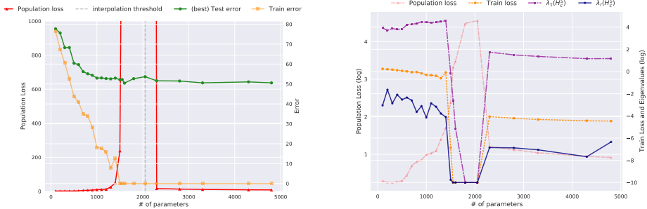
Figure 3: (Left) Double descent curve for CE loss and (right) log-scale plots of the test and train loss, alongside Hessian eigenvalues, for a one-hidden layer neural network trained for 40K epochs.
