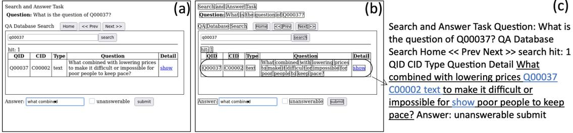
Figure 10: Example of our OCR emulation. (a) Example screen. (b) Detected words. detected words are surrounded by solid boxes. (c) Obtained text sequence. Parts with the broken order are underlined.
