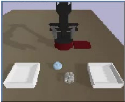
Figure 8: Bin-Sorting task used for our simulated evaluations. The task requires sorting the cylinder into the left bin and the teapot into the right bin.
