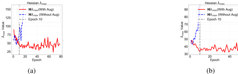
Figure 5: Training dynamic on VGG-small. a and b: Maximum eigenvalue of the Hessian without and with normalization. The dashed vertical lines indicate the epoch at which the non-data-augmented model reached approximately 90% training accuracy.
