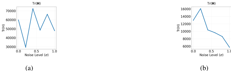
Figure 6: VIT-Base experiment on a subset of ImageNet, trained with SGD ( lr = 1e-4 , momentum = 0.9). We monitor the trace of the Hessian at the end of the first epoch as the variance of injected Gaussian noise increases. a shows the standard model, while b uses per-sample mean-variance normalization applied strictly across all layers.
