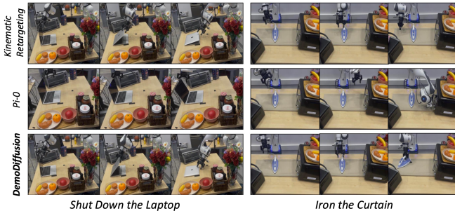
Fig. 4: Qualitative comparisons for real-robot manipulation. Rollout progressions (start, intermediate, final frame) for two tasks. Kinematic retargeting (top) produces plausible motion but loses contact before completing the task. Pi-0 (middle) performs general reaching but fails to manipulate the correct object. DemoDiffusion (bottom) reaches the object and maintains contact through task completion. See project page for full videos.
