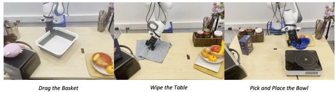
Fig. 8: Zero-Shot Generalization to New Objects. We evaluate DemoDiffusion ’s generalization capabilities to new objects on 3 tasks - drag the basket, wipe the table, pick and place the bowl. While the objects have different colors and shapes from those of objects in the human demonstration, DemoDiffusion adjusts its behavior to these new objects. Please refer to the website for detailed visualizations.
