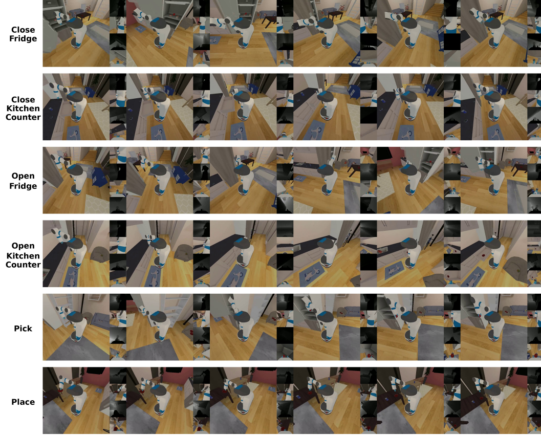
Figure 4: Sample execution trajectories for six household manipulation tasks in ManiSkill-HAB evaluation. Each row shows a temporal sequence of frames for a different task performed by AuxVLA. For each timestep, the large image shows the third-person view of the robot and environment, while the four smaller inset images display the multi-modal sensory inputs used by the model: head depth, head RGB, hand depth, and hand RGB observations (arranged vertically from top to bottom).
