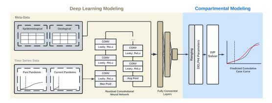
Figure 1: **Model Architecture of HG-DCM** HG-DCM consists of two parts: deep learning modeling and compartmental modeling. The deep learning modeling part predicts the compartmental model parameters, and the compartmental modeling section uses the predicted parameters to construct the predicted cumulative case curve for the pandemic.
