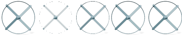
Figure 7: Models recovered from different regular geometry representations under various volume resolutions. From Left to Right : Original, TSDF with K = 64 , TSDF with K = 128 , TSDF-Def with K = 64 , and TSDF-Def with K = 128 .
