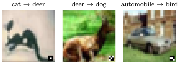
Figure 4: Examples of backdoored CIFAR-10 images with triggers. The trigger is a 3 \times 3 black/white random pattern placed at the bottom-right corner. This causes the model to misclassify the image to the corrupted class.
